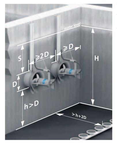
The following guidelines can be used to determine the minimum distances for this type of pump installation. Should your conditions differ please contact your Xylem representative for a satisfactory solution.
