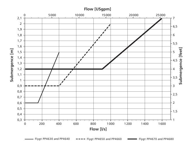
In tanks that are shallow or have poor inflow conditions, it may be impossible to provide the amount of submergence specified in the guidelines above. In such cases, the pump can be equipped with a vortex protection shield. Such shields are designed to reduce the tendency to form vortices and swirl and to make it possible to operate with less than the prescribed submergence.
