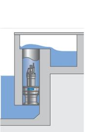
In concrete structure: For pumping to channel. No check valve is required.
