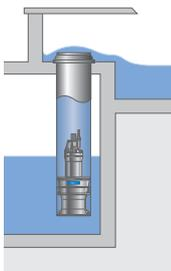
In manufactured column: For pumping to channel. No check valve is required.
