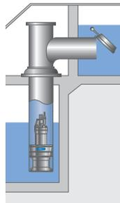
With submerged outlet and flap valve.
