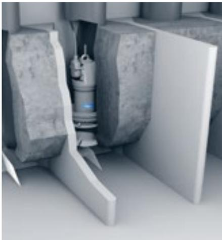
The Flygt PL 7000 range transports medium to large volumes at low heads. The submersible IP 68 motor and slim Propeller hydraulic provides a considerably smaller footprint than non-submersible pumps, enabling compact, low-cost pumping stations which do not require any superstructure.
